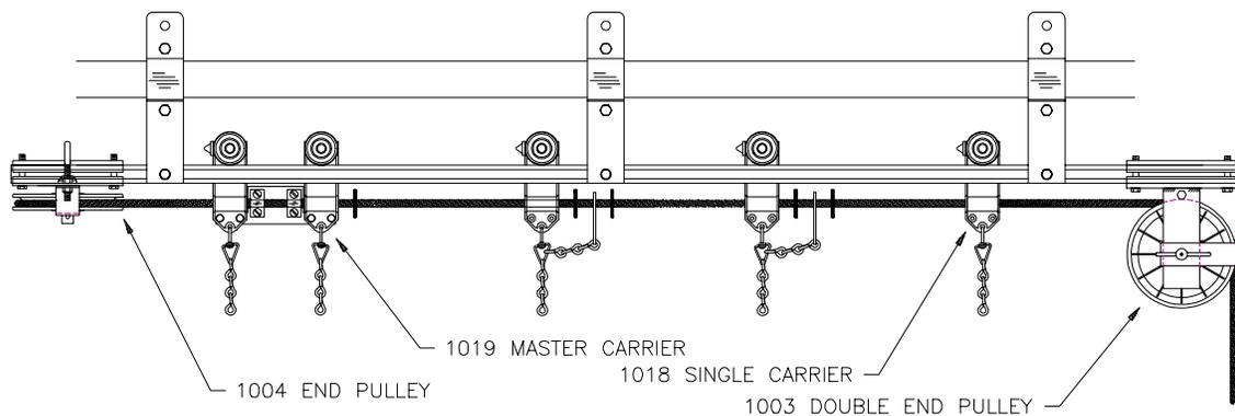
Model No. 1018 Heavy Duty Straight Track was developed especially for use in television studios where an exceptionally quiet, heavy duty track is desired. Equipped with neoprene-tired ball bearing carriers and neoprene bumpers to insure the quietest operation available in a stage track. Track also furnished with rear fold guides which enable curtain to fold at offstage edges during operation. Track sections available in 10 and 20 foot standard lengths.
