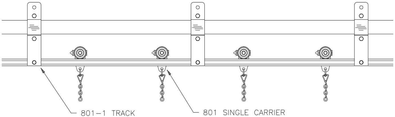
The 800 Series Cyclorama Track is especially suited for use in large television studios. Equipped with neoprene-tired ball bearing single carriers and neoprene bumpers to insure quiet operation. Track available curved to a minimum radius of 4 feet and in straight sections. Track sections available in 10 and 20 foot standard lengths.
