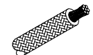
No. 215 BLACK OPERATING CABLE 3/16" diameter black polyester jacket braided over 3/32" galvanized aircraft cable.
