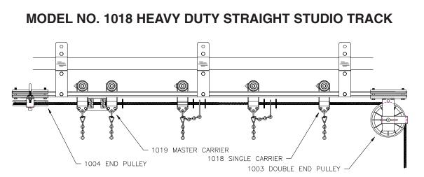
Model No. 1018 Heavy Duty Straight Track was developed especially for use in television studios where an exceptionally quiet, heavy duty track is desired. Equipped with neoprene-tired ball bearing carriers and neoprene bumpers to insure the quietest operation available in a stage track. Track also furnished with rear fold guides which enable curtain to fold at offstage edges during operation. Track sections available in 10 and 20 foot standard lengths.
