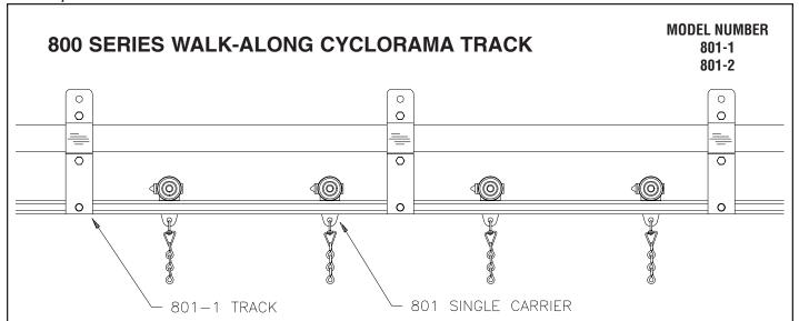
The 800 Series Cyclorama Track is especially suited for use in large television studios. Equipped with neoprenetired ball bearing single carriers and neoprene bumpers to insure quiet operation. Track available curved to a minimum radius of 4 feet and in straight sections. Track sections available in 10 and 20 foot standard lengths.
